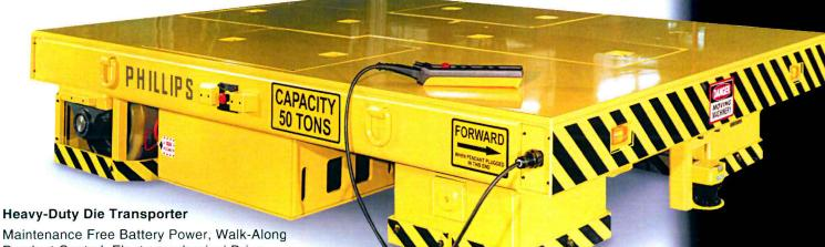
Maintenance Free Battery Power, Walk-Along Pendant Control, Electromechanical Drive and Steer, Optional Laser Scan Bumpers.
